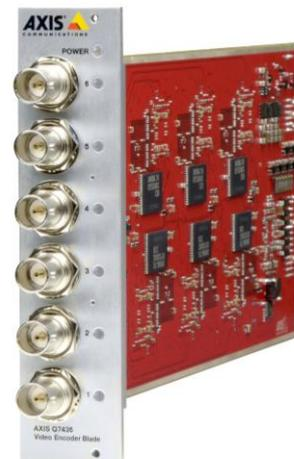
*AXIS Q7436 Video Encoder Blade is a 6-channel encoder blade with support for 60/50 fps.*
