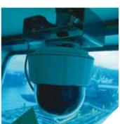
A stabilizer (ballast) has been installed between the AXIS P5532 camera set up in the pilothouse, and the ceiling, avoiding adverse influence from hull vibrations.
